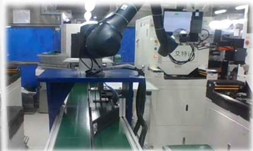
Mobile Phone Testing using Vision - Foxconn
