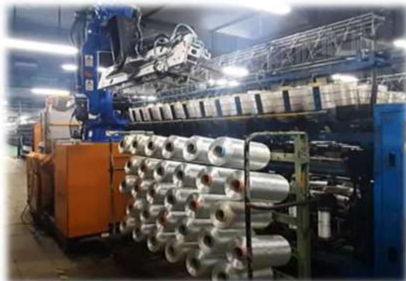
Vision based Bobbin Pick and Place - SRF
